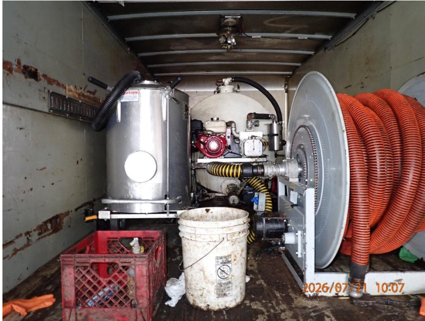
Grease pump truck
